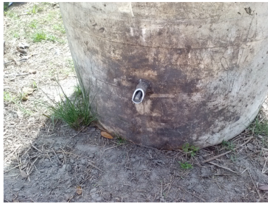
Water nipple installed in drum
